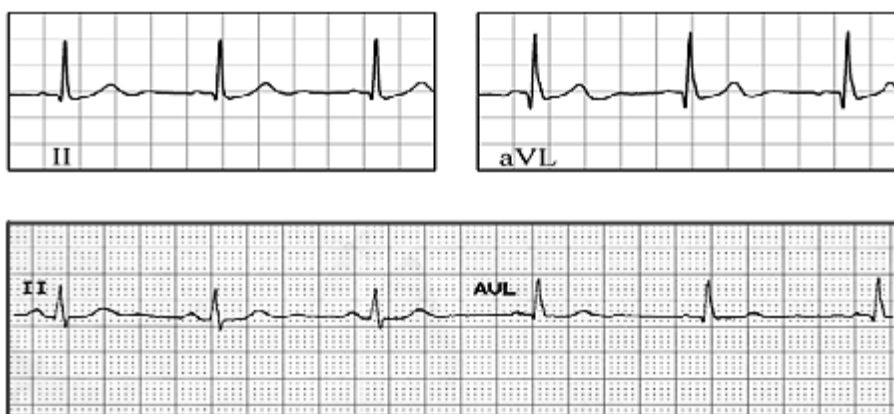
Comparison of two vectors from a pair of EPIC sensors (top) and two conventional Ag/AgCl electrodes (bottom)
