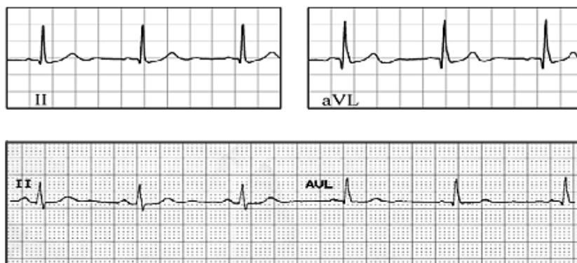
Fig. 4 Comparison of two ECG vectors from a pair of EPIC sensors (top) and two conventional Ag/AgCl electrodes (bottom)
