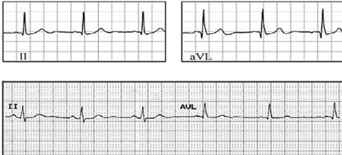
FIGURE 5. ECG READOUTS SHOWING THE RESULTS USING EPIC (TOP) VS. TRADITIONAL WET ELECTRODE ECG (BOTTOM)
