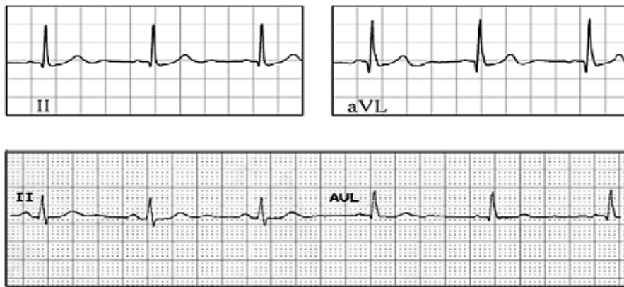
Fig. 4 Comparison of two ECG vectors from a pair of EPIC sensors (top) and two conventional Ag/AgCl electrodes (bottom)
