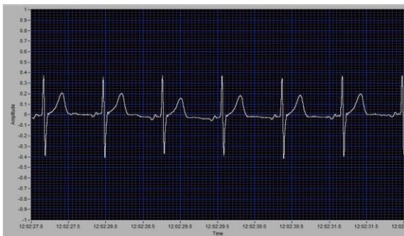
Figure 1: Differential signal from two sensors in contact with the skin showing ECG trace
