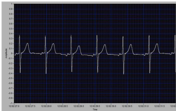
Figure 1: Differential signal from two sensors in contact with the skin showing ECG trace
